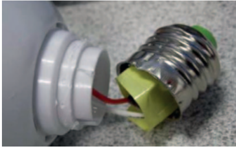
Fig 6. Example of where body of LED lamp has separated from lamp cap when force representative of that required for lamp replacement is applied allowing access to live parts
