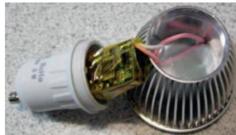
Fig 5. Example of LED lamp that can be easily disassembled to allow access to live parts
