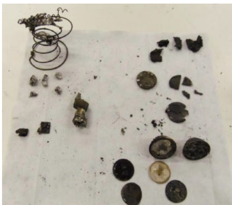
Fig 7. Parts of damaged LED lights found within the remnants of a bed deemed to be the source of fire that resulted in a fatality. Note the remains of an aluminium heatsink melted onto one of the mattress springs. Image courtesy of London Fire Brigade.
