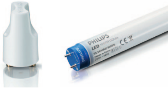
Fig 9. Example of LED tube and replacement for starter switch that may be used to replace a fluorescent tube in a switch-start fluorescent fitting. Images courtesy of Philips.
