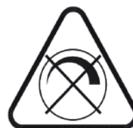
Fig 16. Symbol that lamp is not suitable for use with a dimmer switch.
